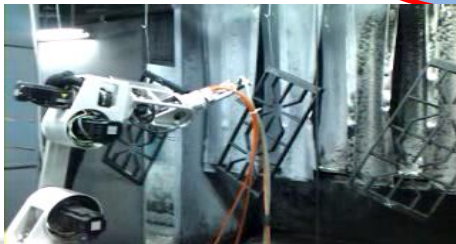
Stove parts sand blasting
